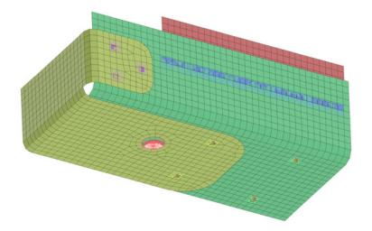
Fastenings such as bolt connections, adhesives and spot welds are automatically changed to reflect any design alterations to the vehicle.
