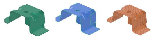
**3D**EXPERIENCE automatically creates a midsurface of every sheet-metal part, then applies a mesh based on rules defined by the user.
