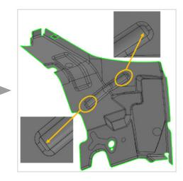
Any issues with the midsurface are flagged so users can check and amend them to ensure 100% accuracy before the mesh is applied.
