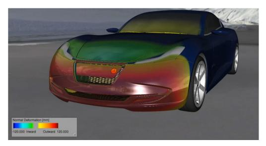
DesignGUIDE connects performance to design using interactive, color-coded surface maps to indicate how style decisions will affect elements such as aerodynamic performance, water management and wind noise.
